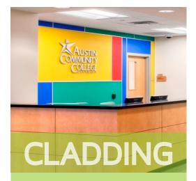
Super thin Lightblocks material is ideal for cladding. Installed flat or cold bent in both fire rated and non fire rated options. The superior durability makes it ideal for cladding of walls in high traffic areas like schools, hospitals, and airports. In the image, you can see our single sided Class A Palette material direct glued to the wall with additional trim hardware.
